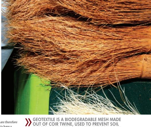
OUT OF COIR TWINE, USED TO PREVENT SOIL EROSION AND KEEP AND BIND THE SOIL UNTIL NATURAL VEGETATION IS GROWING UP IN SLOPES AND BANKS. GEOTEXTILES ARE MANUFACTURED IN VARIOUS EYE SIZES AND CAN BE CUSTOMIZED IN TERMS OF WIDTH AND LENGTH ACCORDING TO THE REQUIREMENT. THE INDUSTRY IS WORKING WITH THE INTERNATIONAL EROSION CONTROL ASSOCIATION (IECA), IN MAINTAIN QUALITY AND TECHNICAL REQUIREMENTS OF THE WORLD MARKET.
