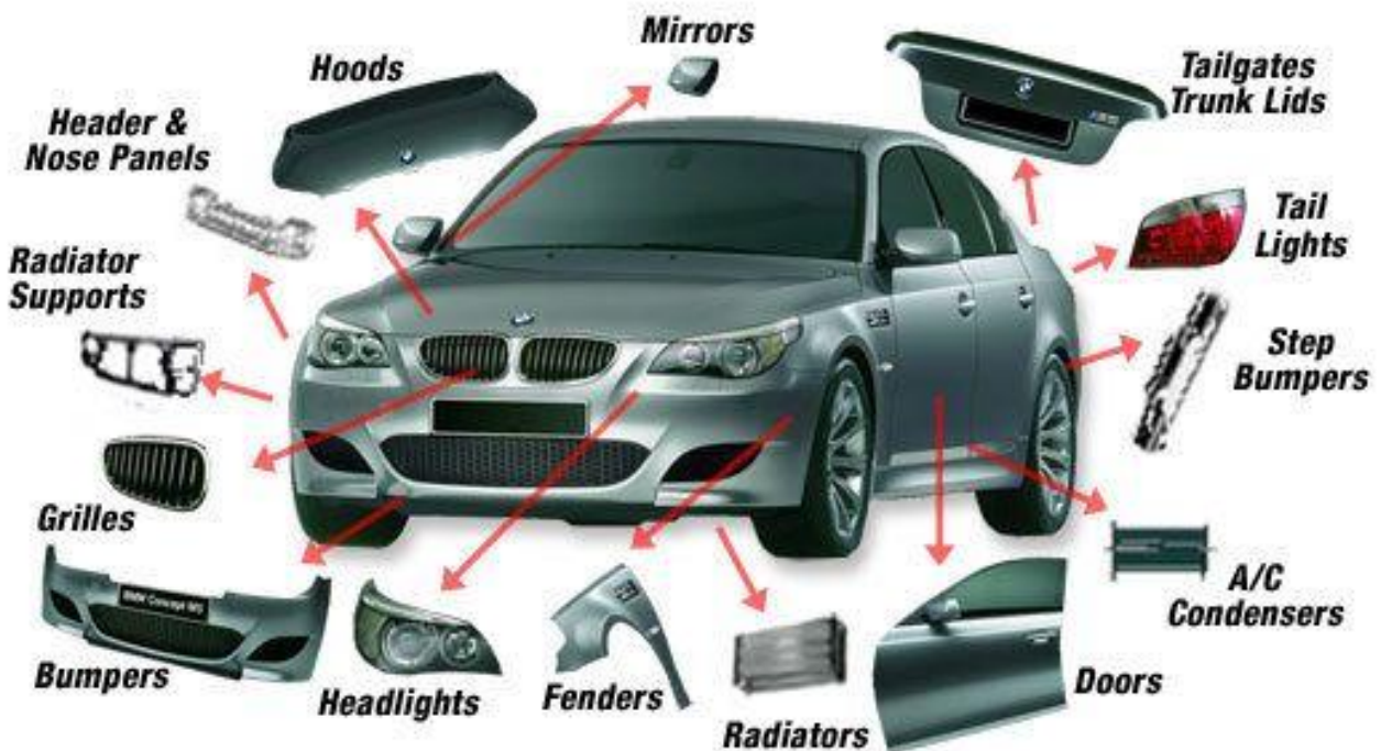
Figure 3 - An exploded view of a car
